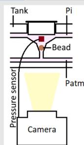
Figure 1 – Fluidic system of compression for microspheres.
